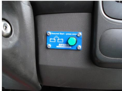
The ASC+ jumpstart automatically and safely creates a 24V jump-start feed from a 12V vehicle at the push of a button.
